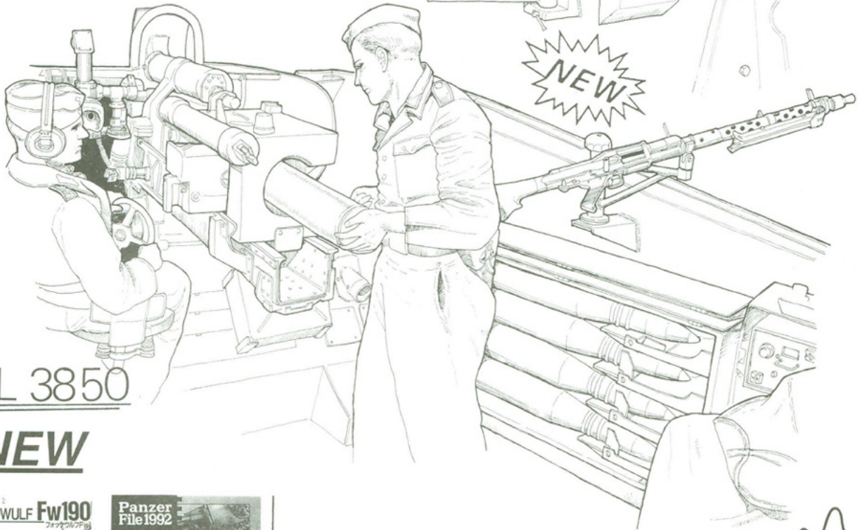
Gun breech and loader's position of 8.8cm Pak43/1.
